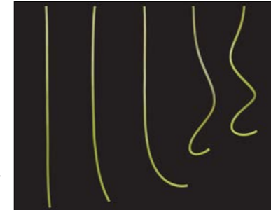
helices and global helices. Given curvature, length, weight and stiffness, their model will predict the shape of a hair, steel pipe or
