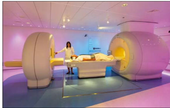
The Philips whole-body PET/MR scanner, which allows sequential PET and MR images to be acquired in the same session. (Image credit: Philips.)
