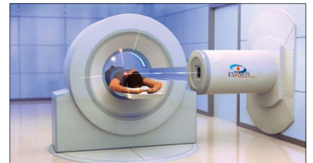
Where physics meets medicine. Artist's view of an in-beam PET device for hadron-therapy monitoring. (Image credit: Nymus3d/ENVISION.)
