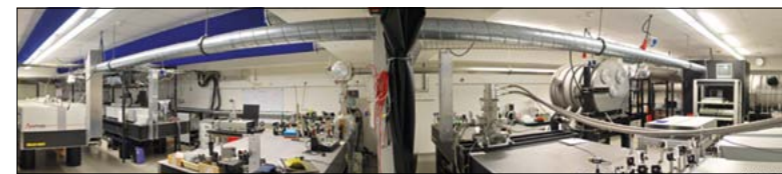
The Arcturus Laser at Heinrich-Heine University Düsseldorf, where two 200 TW beam lines can be used for particle-acceleration studies. (Image credit: T Toncian, University Düsseldorf.)
